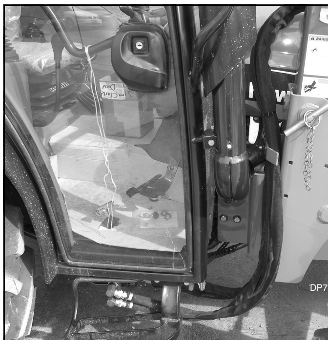
Figure 10. Hydraulic Hose Connection
